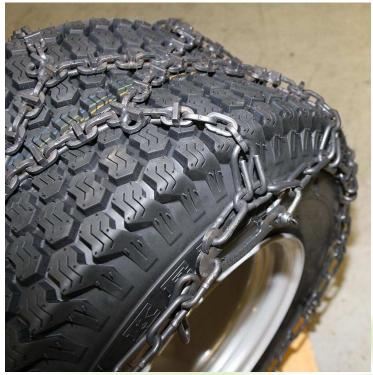
Here also the shackle has been closed with its threaded pin.
