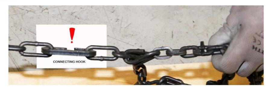
The looking behind the tyre, unite both ends of the chain, using the connecting hook.
