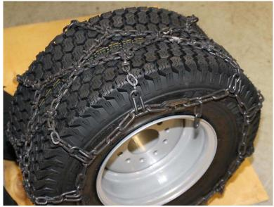
Both the c-shape top linkages connected.
