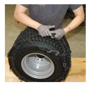
Then pull up the chain, to connect the top of the links, using now the loose c-shape chain links
