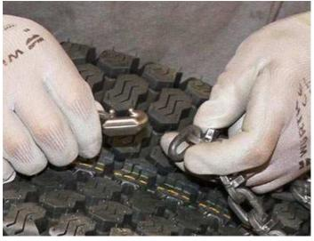
Connecting both ends of the chain, on the top of the tyre, using the separate c-shape linkage.
