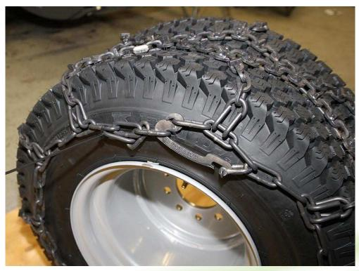
Finally do not forget to tie up the remaining loose chain-links with some cable ties etc.
